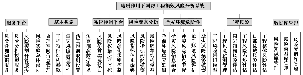
图6 地震作用下国防工程损毁风险分析系统功能模块 Fig.6 Function modules of risk analysis system on earthquake-damaged military engineering
